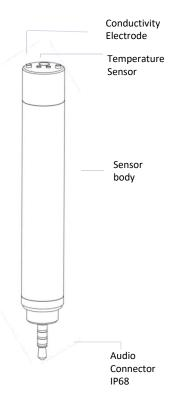
Broadsensor conductivity sensor measures conductivity by AC voltage applied to 316 or C22 electrodes. The sensor requires little maintenance or special attention for storage and can measure high conductivity water long-term.
